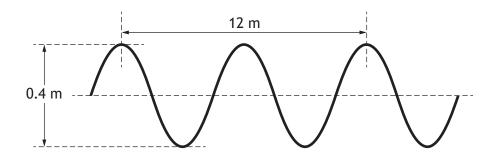
The speed of the wave is  $3.0~\text{m}\,\text{s}^{-1}$ .
