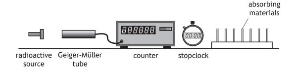
Different absorbing materials are placed, in turn, between the radioactive source and the Geiger-Müller tube, and the count rate is determined.
