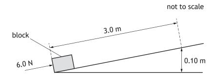
The force of friction between the block and the slope is 2.0 N.
