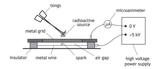
A radioactive source is placed close to the metal grid.
