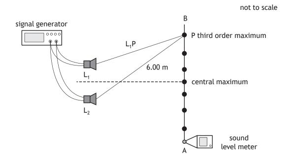
A sound level meter is moved from A to B, and a series of maxima are detected.
