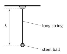
A long string has a steel ball attached to the end of it. The length L of the pendulum can be adjusted.
