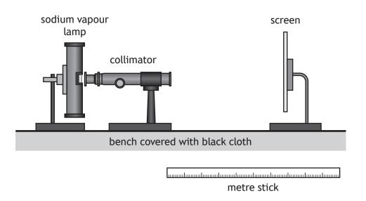
(a) The parallel beam is shone onto a screen. The distance between the end of the collimator and the screen is 0.40 m.
