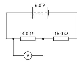
Calculate the reading on the voltmeter. Space for working and answer
