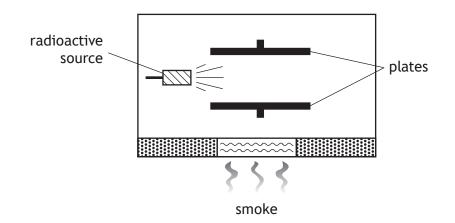
In most smoke detectors the radioactive source used is americium-241, which emits alpha particles.
