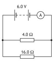
(i) Calculate the total resistance of the circuit. Space for working and answer
