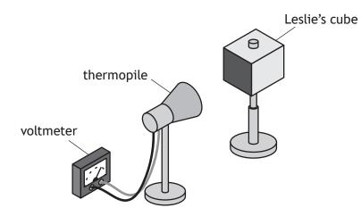
The student fills the cube with hot water and measures the amount of infrared radiation at different distances from the cube, using the thermopile.
