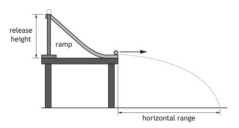
(a) The student releases a marble from different heights on the ramp and measures the horizontal range.
