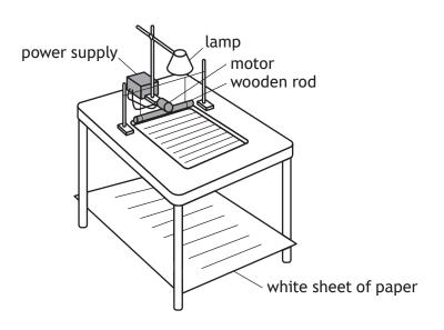
The wooden rod moves in and out of the water to generate water waves.
